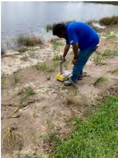
Tuesday, June 6, 2023 Universal Testing Compaction Test Lake 45
