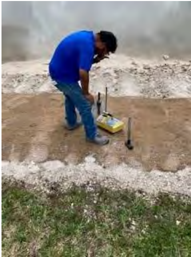
Tuesday, June 6, 2023 Universal Testing Compaction Test Lake 45
